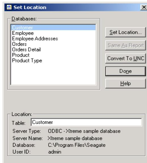
In the example above you will notice that the Set Location Window provides you with the first 3 database credentials for the report. The "ServerName" represents the name of the ODBC DSN for the report. The name of the database is located next to the "Database:" line. As well the UserID for the database is stored next to the "UserID:" line. It is a good idea to record this information, as it will be the same information that you will later need to provide in your ASP code.
